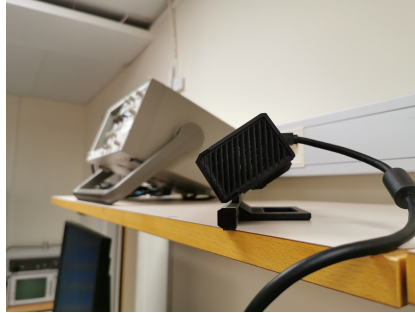
Fig. 2: Placement of Kinect camera in Test-Environment on a shelf facing downwards toward the ground to allow for a maximized field of view.
