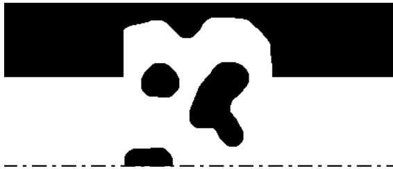
Figure 3.7: Optimized design that only allows uni-directional acoustic flow (left to right) for frequency range 8–9 kHz
