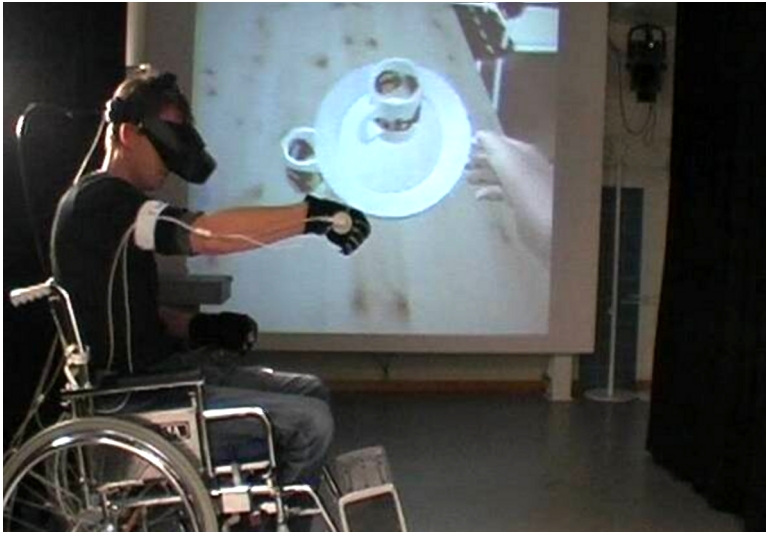
Figure 1.1: Classical full-fledged VR-setup, with motion-tracked head-mounted display (HMD) and tracked, grip-sensitive, gloves. In this application the user can move around freely in the world by turning the wheels of the wheelchair. Hands are represented in the virtual world and can be used to grab and move objects with simulated physical properties. The head is motion-tracked with six degrees of freedom, allowing the user to look around freely by moving the head, for example, to look under the table. This image is from an earlier VR-project in our lab.
