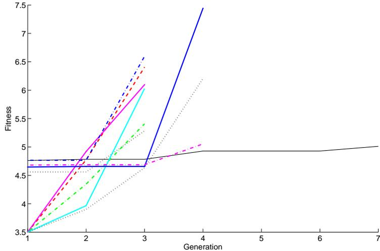
Figure 8: Maximum path fitness in a population as a function of generation, for ten different problems solved by the genetic algorithm. When the fitness value becomes at least 5, the path is considered traversable and search is terminated.
