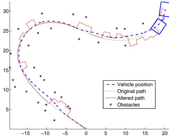
Figure 7: The result of replanning a path. The figure shows the original path as well as the replanned one, and the vehicle's position as it tracks the new path. The vehicle is shown in its final position.
