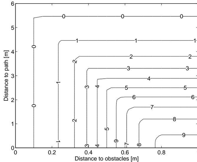
Figure 4: Level curve for the fitness function used for path search. The fitness value is a function of the vehicle's shortest distance to any obstacle and its distance to the original reference path. If the fitness value is 5 or above, the path is regarded as traversable at this particular point. An entire path is regarded traversable if all points the vehicle passes through in path-tracking are traversable.
