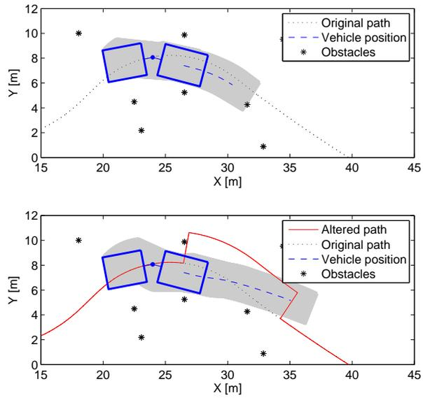
Figure 3: If the simulation predicts a collision with an obstacle, as in the upper figure, the path is replanned such that the obstacles are avoided, as shown in the lower figure. The figures show the original position of the vehicle and the area it would cover while tracking the path (the gray area). In the lower figure, the altered replanned path can be seen as well.
