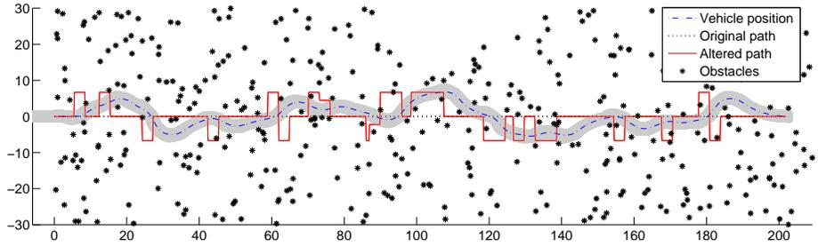
Figure 9: A totally new path can also be planned, given only the start and goal points. In this example, a random set of obstacles is generated. The original path is a straight line between the start and goal points. The vehicle is allowed to drive at most 10 meter away from this path and no closer than 0.5 meter to any obstacle.
