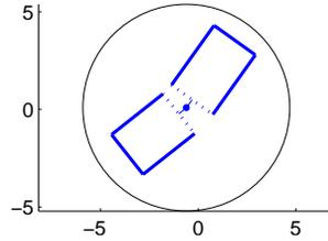
Figure 5: To speed up the computation of the smallest distance between obstacles and the vehicle, only the continuous lines in the figure are used. The dotted lines can never be closest to an obstacle due to the the vehicle’s geometry, unless a collision was detected in a previous time step. Furthermore, only obstacles within the bounding circle drawn around the vehicle are considered in the computation.
