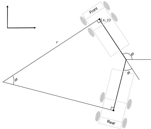
Figure 10: Definition of steering angle  $\phi$ , position  $(x, y)$ , heading  $\theta$ , and turning radius  $r$  for an articulated forest machine. The global coordinate system for the pose  $(x, y, \theta)$  can be seen in the upper left part of the figure.
