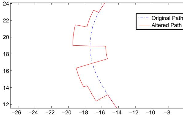
Figure 2: 10 meters of the original path in front of the vehicle are divided into 5 segments. By offsetting each segment perpendicular to the original path the search function tries to find a combination of offsets that allow the vehicle to avoid the obstacles.
